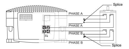
Figure 2.3.2: 8 Lead Motor Series Connections
